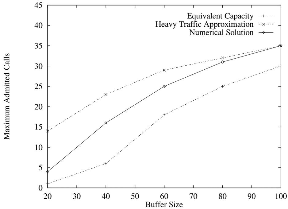
Figure 12: Variation of the maximum number of class 1 calls with buffer size – required cell loss probability =  $10^{-6}$
