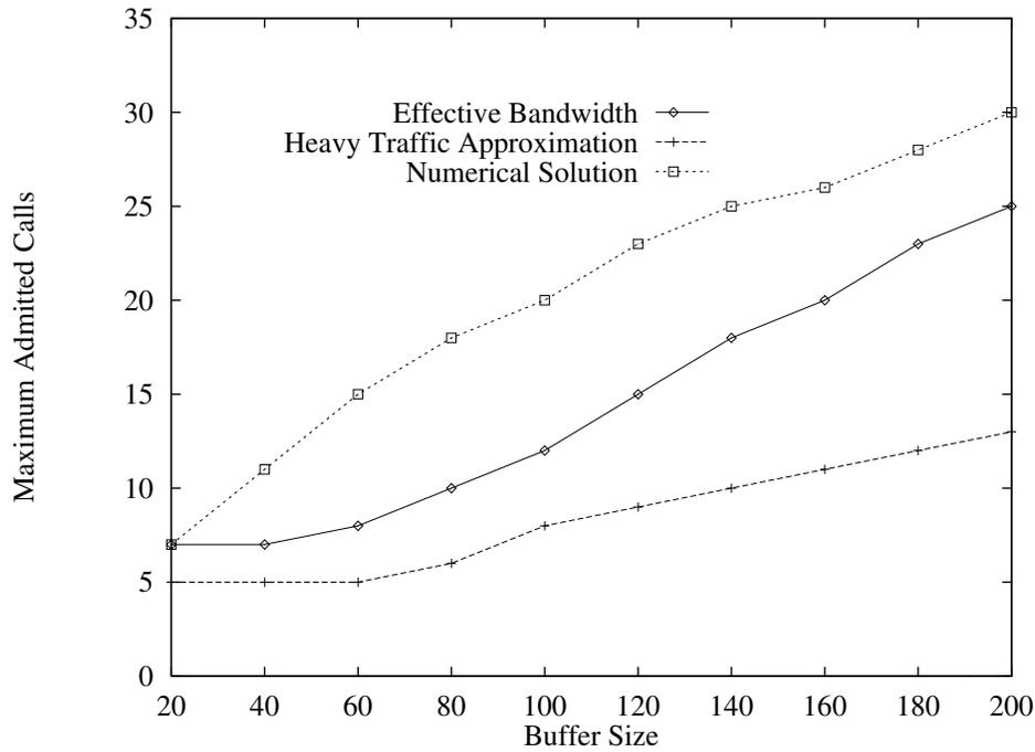
Figure 10: Variation of the maximum number of calls with buffer size – required cell loss probability =  $10^{-6}$
