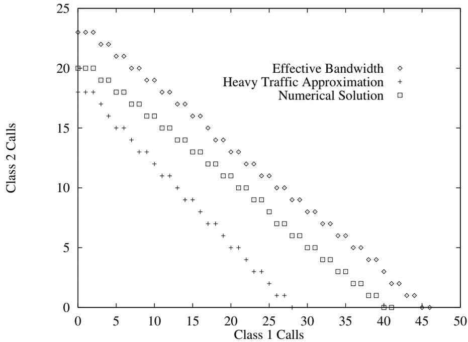
Figure 8: Admission regions for the CAC methods as compared with numerical solution
