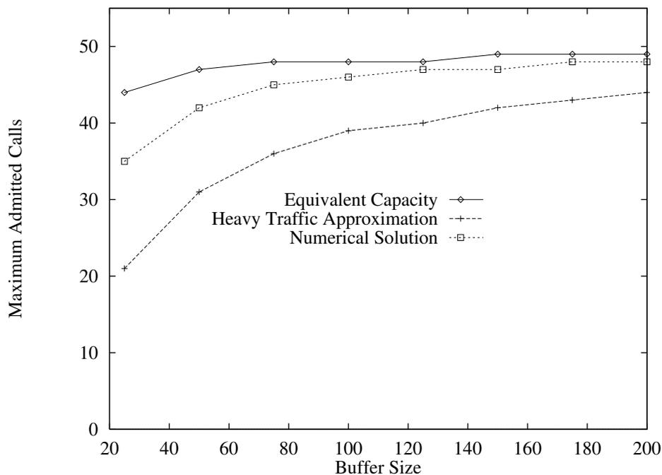
Figure 9: Variation of the maximum number of class 1 calls with buffer size – required cell loss probability =  $10^{-6}$
